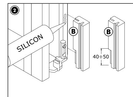
Trim the lower position of the vertical pocket jamb **(B)** to accommodate the guide and attach to both sides of the pocket entrance using 4/5 blobs of silicon.
