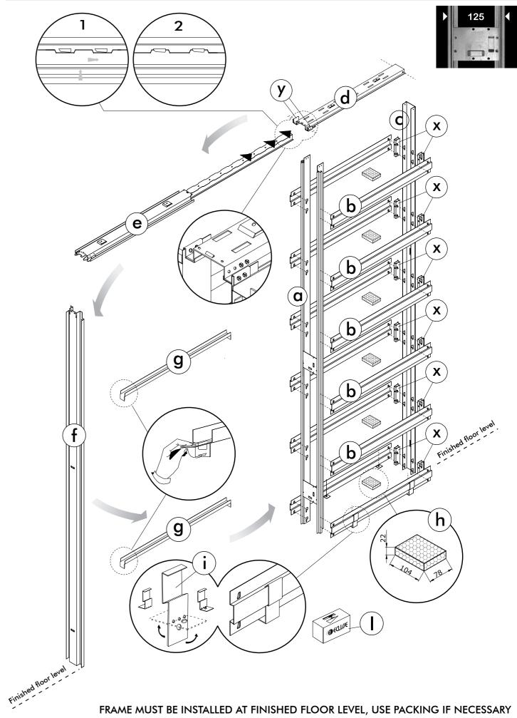
FRAME MUST BE INSTALLED AT FINISHED FLOOR LEVEL, USE PACKING IF NECESSARY
