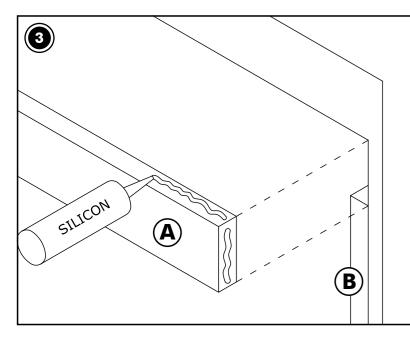
The top horizontal jamb **(A)** needs to be cut to size. Note the rebate on both ends is used to match the top of each of the vertical pocket jambs **(B)**. Fix into place using silicon or if preferred pin or screw into place.
