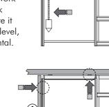
STEP 12 Attach the frame to the studwork by screwing through the vertical (c), metal doorpost (f) and top beam with track (e) ( use ONLY the larger holes so that the screw head goes through the track and locates the top beam). Screw the internal pocket-to-floor brackets to the floor.
