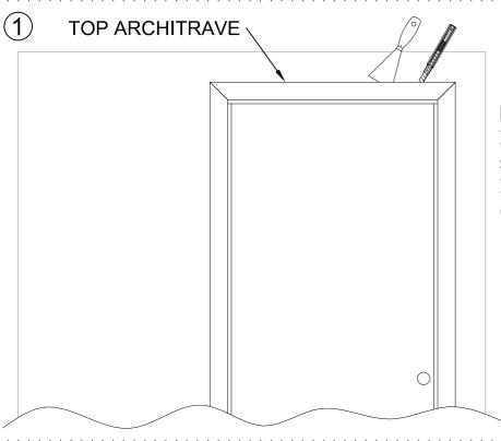
Remove top architrave. If attached with silicone use a spatula or cutting knife. If pin-nailed on be more careful not to damage it.
