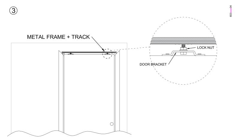
Extend door to almost closed and loosen both lock nuts.
