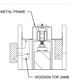
Remove wooden top jamb. If attached with silicone use a spatula or cutting knife. If pin-nailed or screwed be more careful not to damage it.
