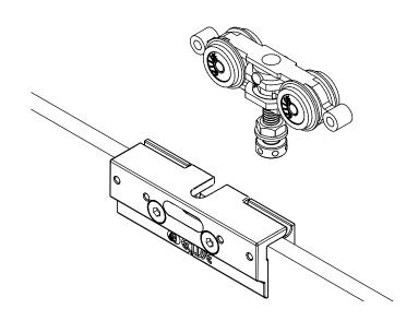
First wind the toothed locking nut onto the capstan headed bolts about half way down, then wind the bolts into the rollers in the top track.
